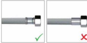
Always check that ferrules are pressed correctly and there are no braiding threads coming out. In case of doubts do not install the flexible hose.
