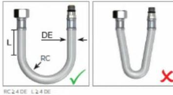
The hoses must maintain a straight section at the connections equal to 4 times the external diameter of the hose (DN6 = Ø 10 mm → straight section 40 mm). The bending radius must not be less than 4 times the external diameter of the hose (DN6 = Ø 10 mm → bending radius 40 mm).
