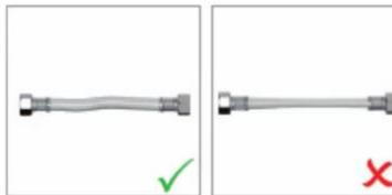
Do not install flexible hoses under twisting or tension conditions.
